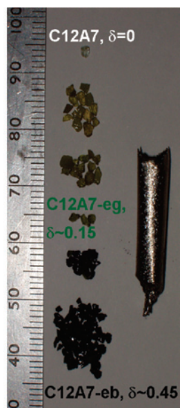
Figure 1. Photograph of mayenite crystals and the titanium container. From top to bottom are shown crystals with increasing electron loadings, and therefore different colors. The single-crystal data were collected for (i) transparent colorless C12A7 (top) and (ii) transparent green C12A7-eg (intermediate) and opaque black C12A7-eb (bottom).
